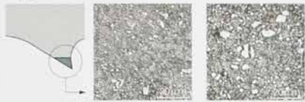
M42 Amada M71 Metallographic picture of edge material
