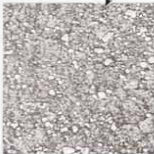
Metallographic picture of edge material (M42 HSS)
